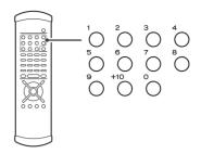
Use the number button to select tracks or chapters for playback. Use the +10 button to enter the first digit of numbers greater than 9 (repeated presses show 1-, 2-, 3- etc.) and the single digit buttons (0 through 9) for the second digit, or single-digit track numbers.
